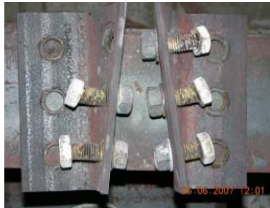
Web cleat connections by Yu et al.
