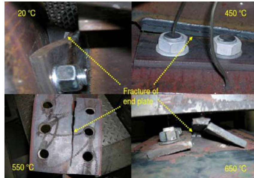
Endplate connections fractured in this robustness project
