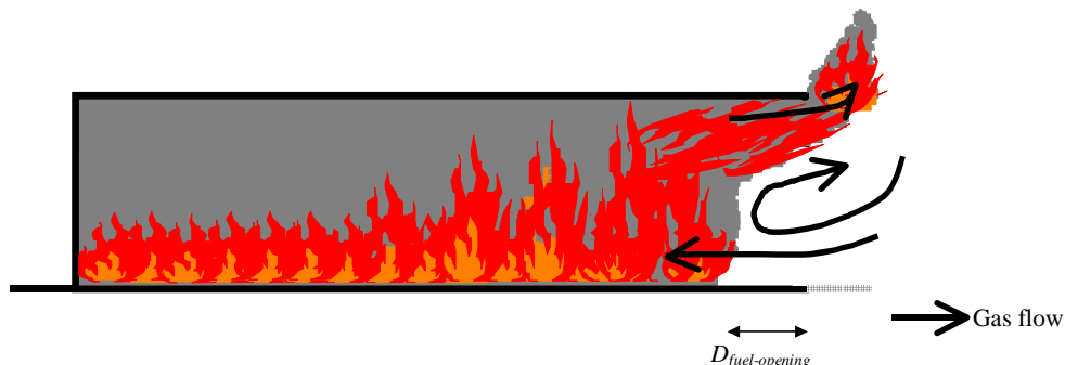
Figure 22 Schematic view of the gas flow through the opening
