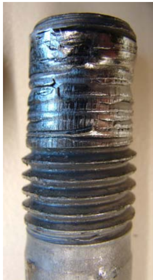
Thread failure at room temperature
